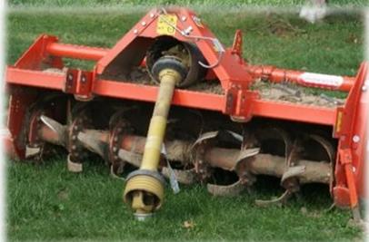
Next up is the rototiller. As you can see, this piece of equipment has big, cupped blades that finely chop the soil. This is the final prep to the bed before planting. The rototiller turns a bed from clumpy dirt to fine, loose soil, great for planting no matter if we are direct seed planting or transplanting cells from the greenhouse.
